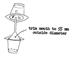
Fig. 2 Transfer method using polyethylene funnel
